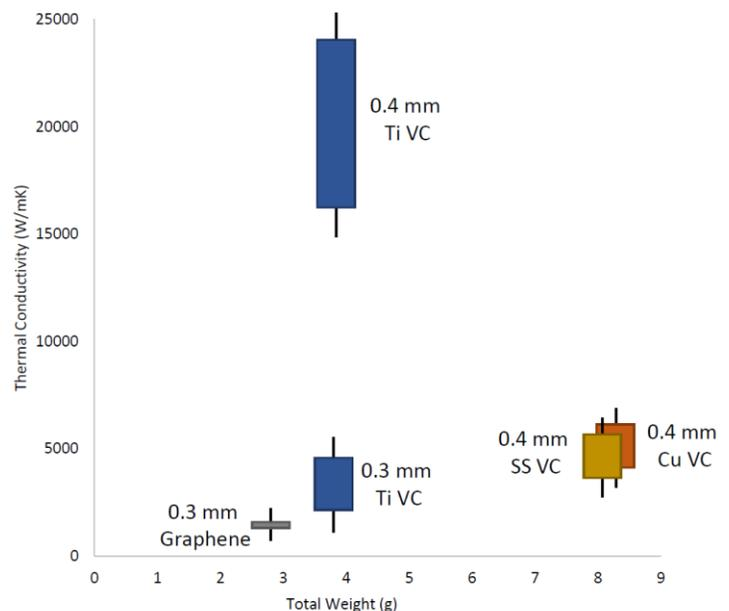
*Represents vapor chamber temperature typical in mobile phones at 60°C.*
