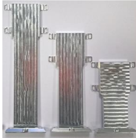
Figure 2: Phase 1 K-Core TMS Single Component (Length= 176.5 mm, 136.5 mm & 96.5 mm respectively)
