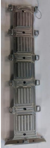
Figure 4: Multi-device k-Core TMS (Mass = 97 g, Length = 176.5 mm)
