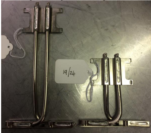
Figure 1: Copper-Water Mini-Heat Pipe TMS's (short & long versions; (Mass = 92 g & 68 g; Length= 176.5 mm & 96.5 mm respectively)
