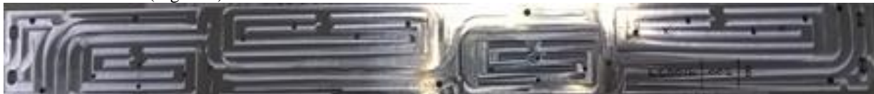
Figure 3: k-Core Chassis Base Embedded Graphite Component (Mass = 171 g)
