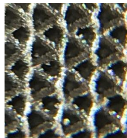
Figure 10: Detailed View of Miniaturised Lattice Cells
