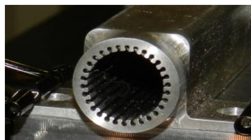
Figure 7: Axially Grooved HP Wick (Aavid)
