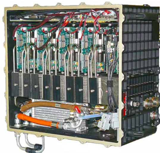
Figure 1. Example rLCS installed in Chassis
