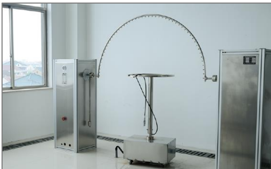
IP Rating (Liquid Ingress) Test Setup Image Source: KLED
