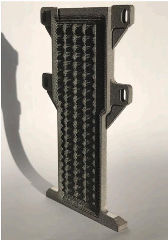
Fig. 8. Titanium-Water AM Vapour Chamber Heat Pipe Capillary Wick Test Piece with Integrated Lattice Structure (Aavid, Thermal Division of Boyd Corp.)
