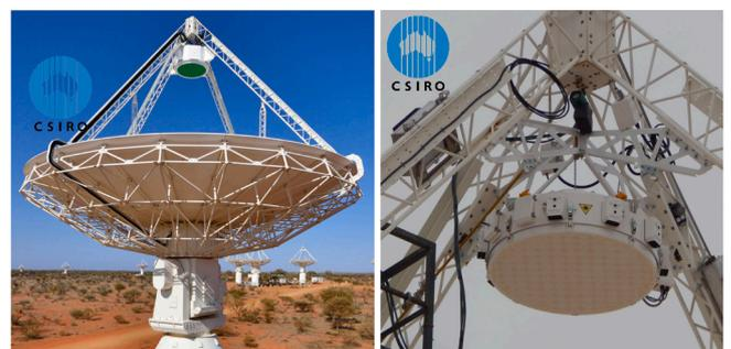
Fig. 10. Photographs of an ASKAP radio-telescope with and close-up view of the PAF receiver module with integrated Aavid UK heat pipe receiver disc (CSIRO).
