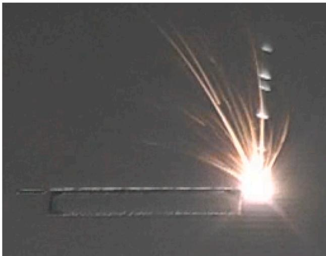
Fig. 1. Manufacture of Aavid AM Titanium Vapour Chamber by Laser Powder Bed Fusion.
