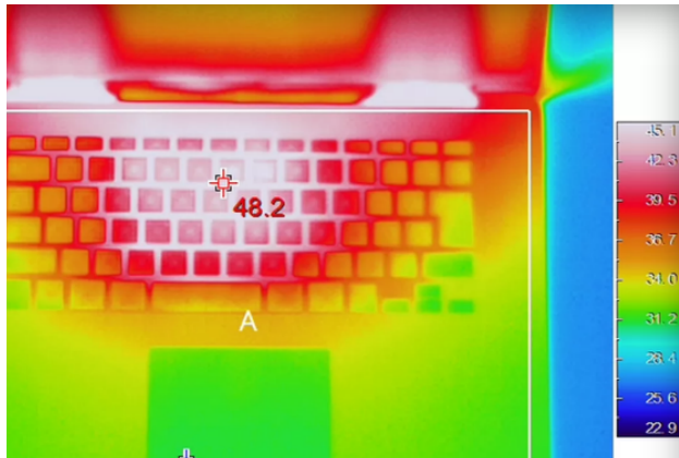
Figure 1. Heat map of a laptop. Source: Boyd Corporation
