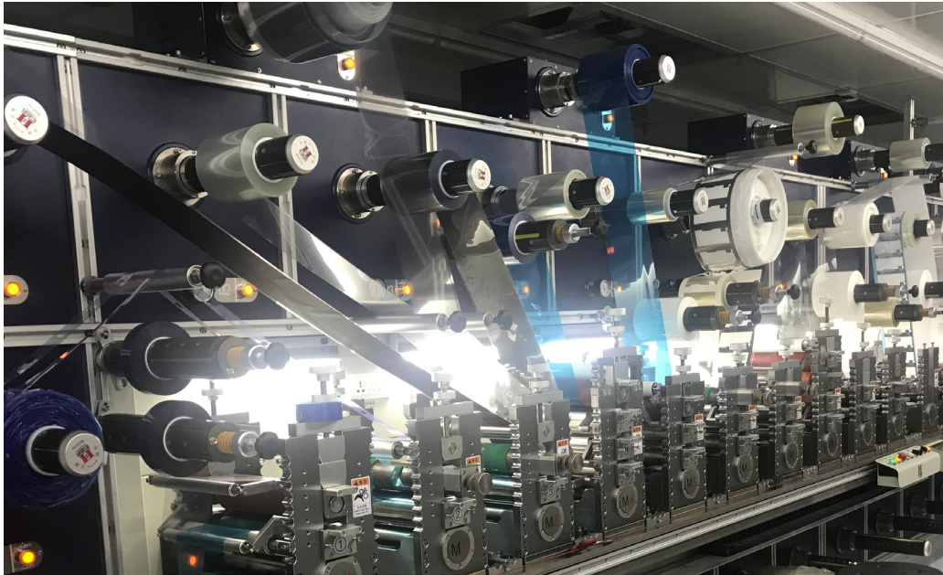
Figure 1: Precision converting of optical films and optically clear adhesives for integrated displays. Source: Boyd Corporation
