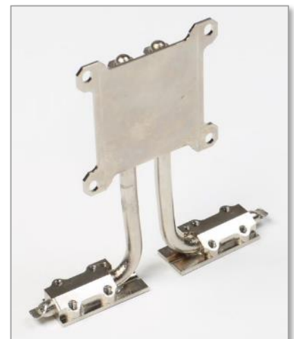
Small Form Factor Heat Pipe Solution
